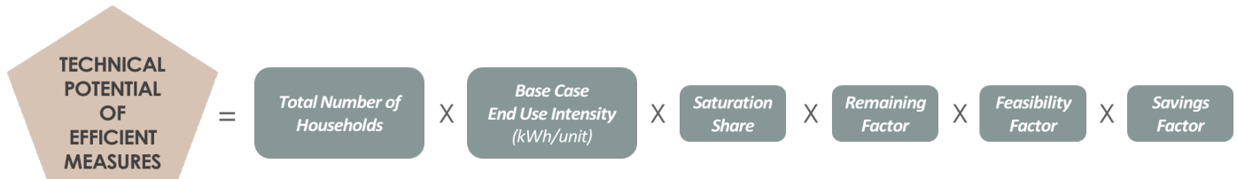
FIGURE 3-3 CORE EQUATION FOR RESIDENTIAL ENERGY EFFICIENCY TECHNICAL POTENTIAL
